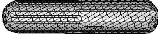
Figure 1. The surface of a (10, 10) finite SWCNT (6 nm in length, 1020 carbon atoms) obtained from the triangulation surface method. The volume is calculated from the Gauss theorem.
